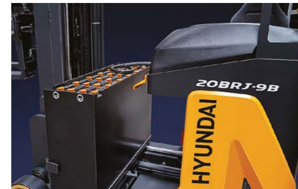
Side battery extraction.
